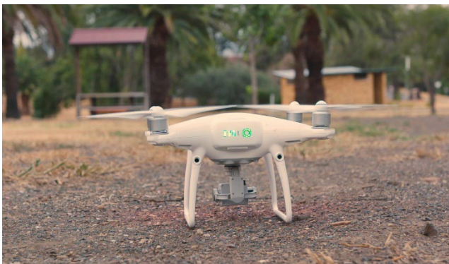
Figure 11 Drones are used to inspect assets as a part of our pre-summer bushfire inspection program
