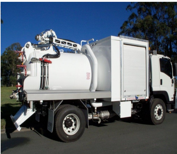
Hydro Excavation Equipment
