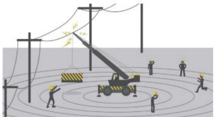
Figure 16: Overhead powerline clearances must be adhered to when operating any mobile plant or equipment, including cranes.
